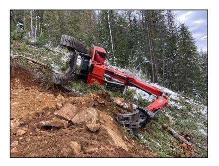
its side. The machine was walking down the slope on the same path it had travelled without incident going up the hill.
