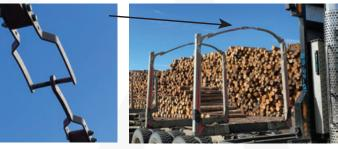
Safety specific aspects of the system include automatic lashing arms, in-cab system monitoring, constant load securement pressure, and remote-control options. The system has been designed to address multiple safety issues including risks to the driver of manual load securement activities to better containment of the load during transport.
