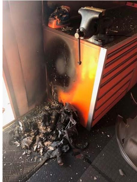
Prevention of spontaneous combustion fires begins with good housekeeping. A clean work area can prevent a fire from spreading and getting bigger by not allowing the fire fuel to burn. Also understanding the potential for self-heating of rags soiled with oils such as linseed oil and turpentine is a key step in eliminating these preventable fires. To properly and safely dispose of oily rags, use the following steps:
