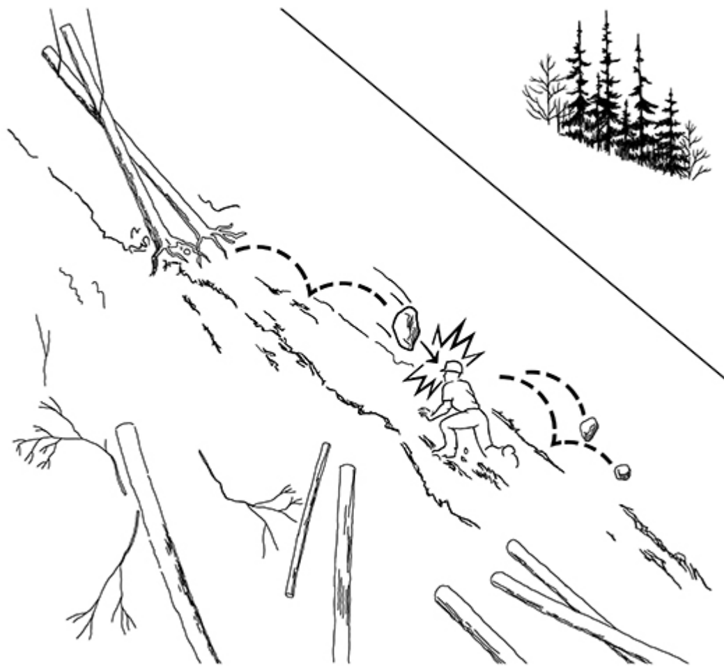
Figure 1: Sketch of hooktender struck by rock as it was dislodged from a root wad
