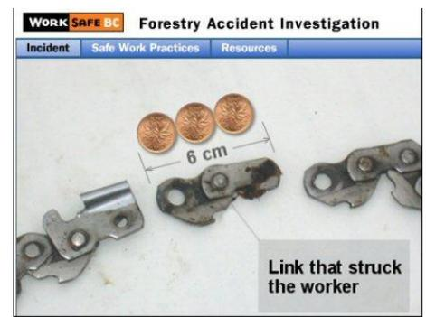
Another worker was using a manual chain saw to cut a dead stump when the chain broke. The broken linkages flew through the air and struck another worker about 35' away. The chain piece removed in life saving surgery had caused injuries similar to being shot by a bullet.
