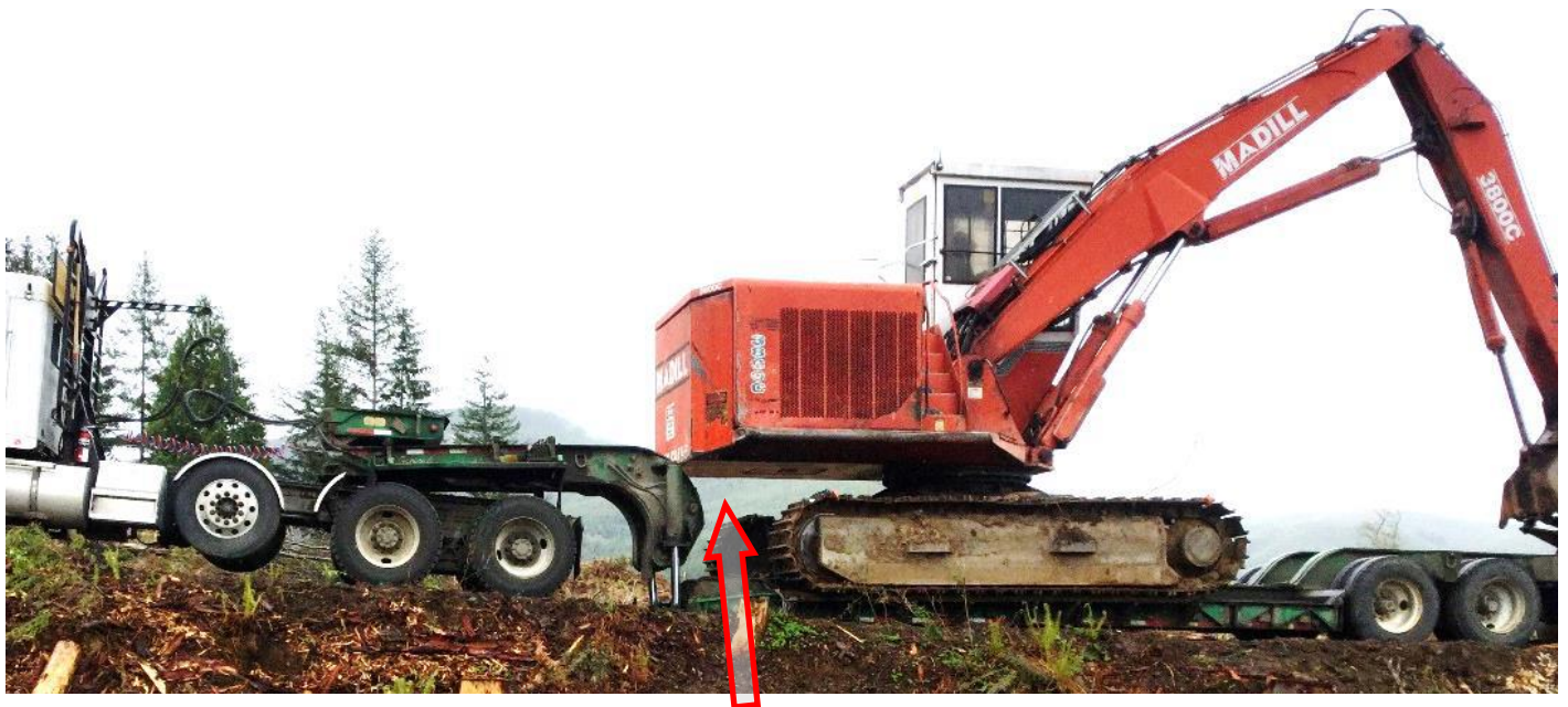
Incident scene showing the position of the operator when the trailer detached from the gooseneck.
